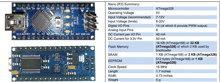
See <u>http://arduino.cc</u> for detailed specifications, overviews, schematics, etc. Core functions, code examples, and links to many of the device libraries can be found in the learning section; refer to the manufacturer's site if using other add-on shields or sensors.
