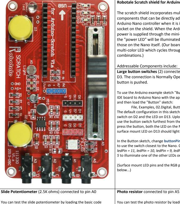
**Robotale Scratch shield for Arduino Nano**
