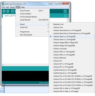
Select the version of Nano from the drop down list in the IDE application. Note that some Nano controllers may use either the ATmega168 or ATmega328 chip on the board (examine the printing on the square IC found on the top of the controller board next to the USB connector. Inland Nano v3 boards should have ATmega328 chips.
